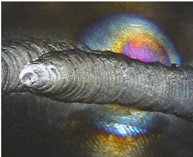
Figure: Endoscope picture, manufacturer's error: seam: insufficient formation before tacking In the picture, blue and brown tempering colours are visible at one point. This error pattern is typical for a manual tack-weld to fix the position of the tube connection without having a sufficient level of protective gas.
